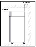
5- To avoid vibrations, the unit must be level.
